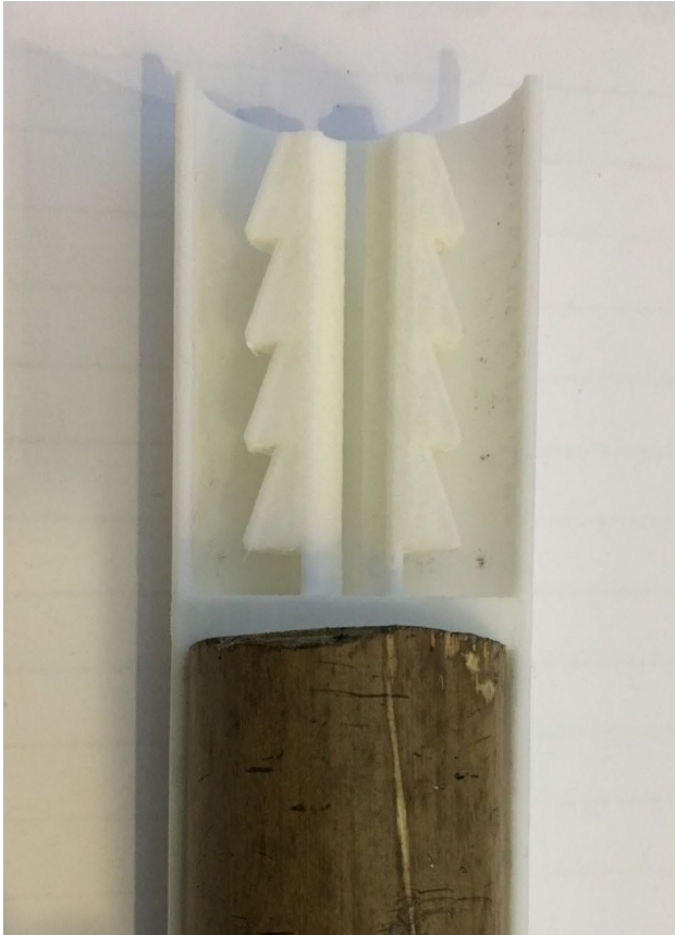
Typical detail to create continuity between the poles in the gridshell.
